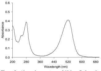
Figure 2 : Absorption spectrum of 10.0 mg/L dye solution at pH 7 ( $\lambda_{max} = 528$  nm).
